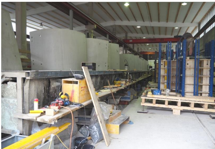
Picture 1 – 3: Production of concrete shells (4 cm thick) for an ice channel of a bobsleigh track.
