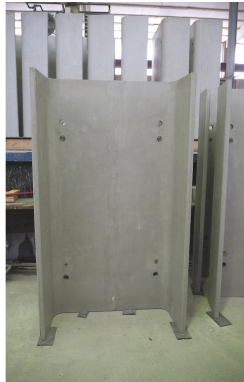
Picture 1 – 3: Production of concrete shells (4 cm thick) for an ice channel of a bobsleigh track.
